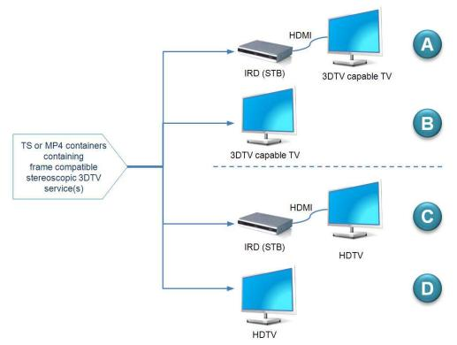
Figure 16: Frame compatible plano-stereoscopic 3DTV IRD use cases
