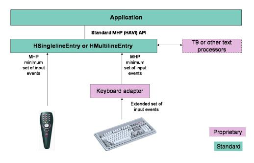
Figure 5: Text Entry Layering Schematic
