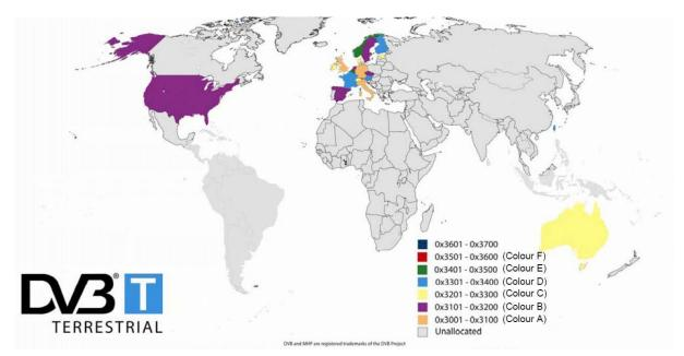
Figure 15: Colour map for allocating network\_ids in terrestrial networks
