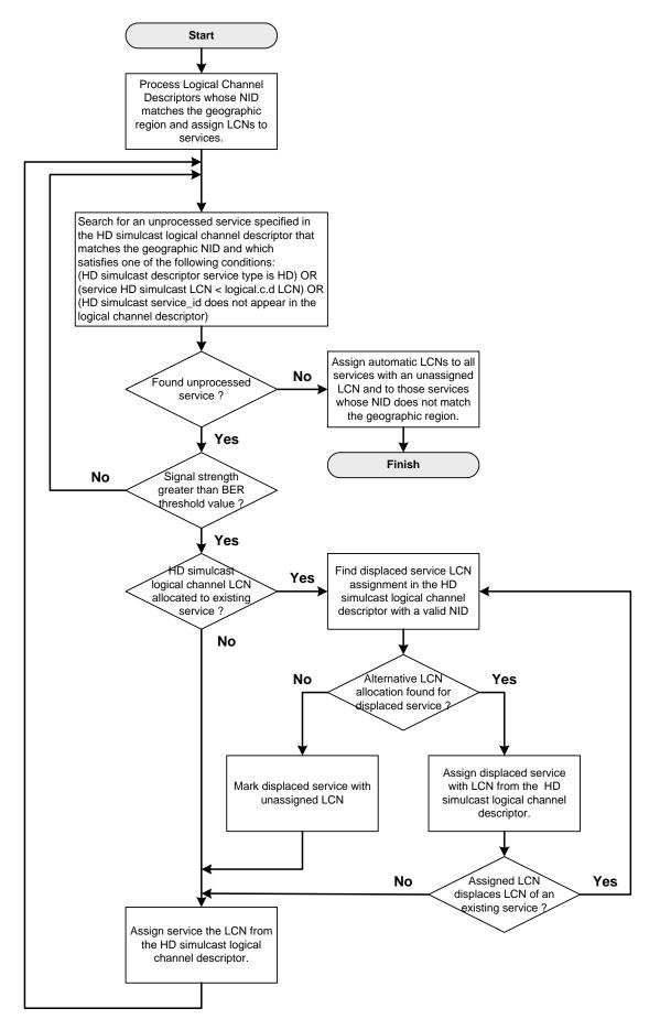
Figure 6: HD\_simulcast\_LCN operation
